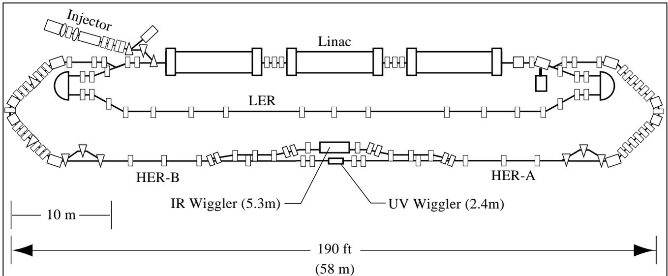
**Figure 1.** Overview of FEL Driver Accelerator, showing 10 MeV injector, 96 MV linac, low-energy recirculation transport (LER) for 105 MeV beam, and high-energy recirculation transport (HER-A) which takes 200 MeV beam to the UV or IR FEL wiggler and returns it to the Linac for energy recovery (HER-B).
