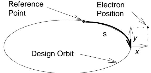
Figure 1. The coordinate system of the storage ring.
