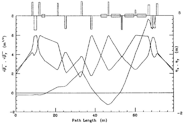
**Fig. 2** The lattice functions of one sextant of the new Accumulator lattice obtained by varying the focusing strength.
