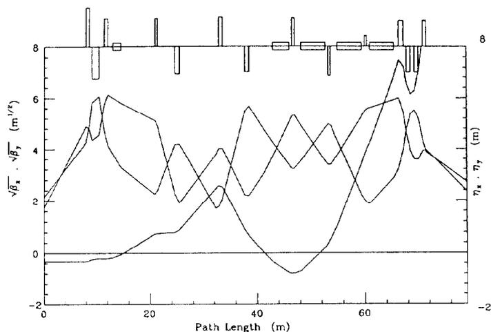
**Fig. 3** The lattice functions of one sextant of the new Accumulator lattice obtained by changing positions of quadrupoles and varying their focusing strength.
