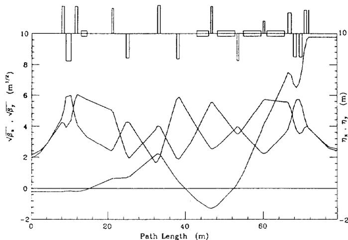
**Fig. 4** The lattice functions of one sextant of the new Accumulator lattice obtained by adding one new quadrupole and varying the focusing strengths of small quadrupoles. The large quadrupoles are not changed.
