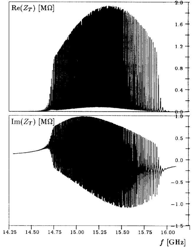
Figure 2: Transverse impedance in the detuned structure
