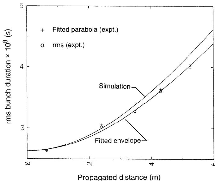
Fig. 1. Bunch length vs. distance propagated for a bunch with initially parabolic shape. Data from an r,z WARP simulation is plotted, as the top curve, on the same axes as experimental measured points, as well as, an envelope solution fitted to the expansion data.
