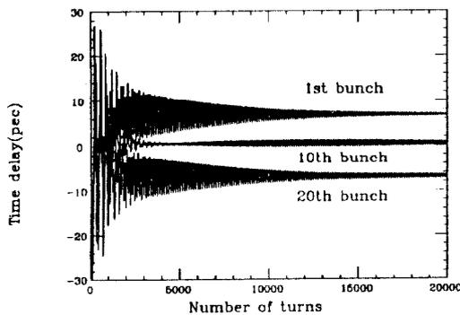
Fig. 3, Time delay from nominal positions of 1st, 10th and 20th bunches in a train versus number of revolution.
