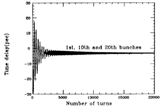
Fig. 7, Time delay from nominal positions, 1st, 10th and 20th bunches in a train for case (a) with passive sub-RF.
