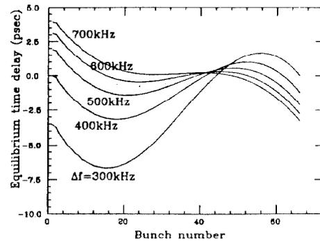
Fig. 8(b) Equilibrium positions of bunches vs. bunch number for case (b) with passive sub-RF.
