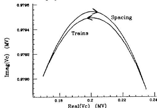
Fig. 2, Trajectory of cavity voltage on complex plane.
