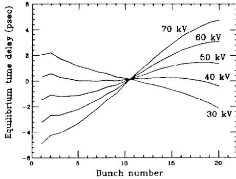
Fig. 6(a) Equilibrium positions of bunches vs. bunch number for case (a) with active sub-RF.
