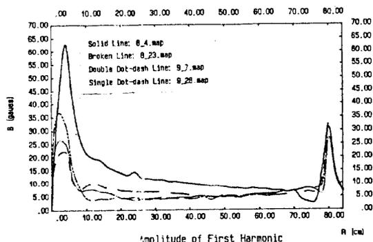
Fig. 7 The improving process of the first harmonic after 4 times of the iteration
