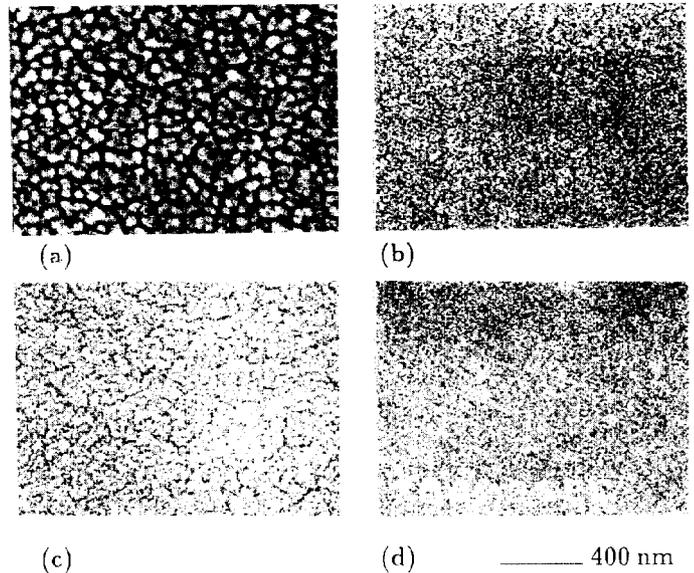
Fig.1 Plan-view SEM images of porous silicon samples before and after RIE. (a) and (b) P-type (100), 0.01 Ω cm, anodization current density is 40 mA/cm<sup>2</sup>, (a) after 2 min RIE, (b) before RIE. (c) and (d) N<sup>+</sup>-type (100), 0.001 Ω cm, 75 mA/cm<sup>2</sup>, (c) after 1 min RIE, (d) before RIE.
