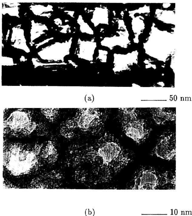
Fig.2 Plan-view TEM images. (a)  $N^+$ -type porous silicon lift-off sample, 0.001  $\Omega$  cm, near lift-off side. (b)  $P^+$ -type porous silicon, 0.001  $\Omega$  cm, anodization current density: 60mA/cm<sup>2</sup>
