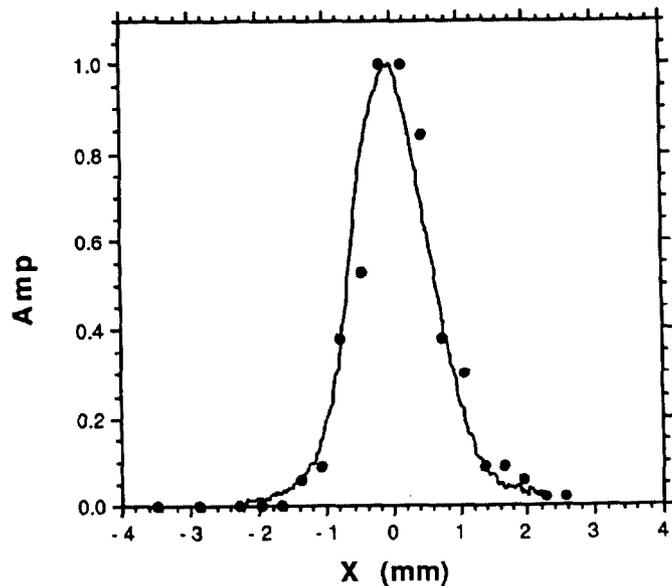
Figure 4. Narrow beam profile measured by the flying wire (dots) compared to the profile measured by the OTR screen (solid curve).
