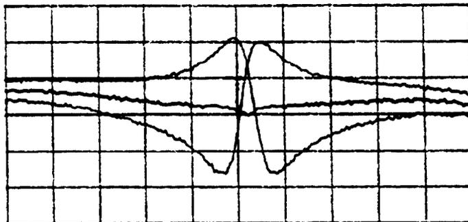
Fig. 2 Transmission through cavity at the  $E_{110}$  null and at  $\pm 1\mu\text{m}$  either side. Vertical 2dB/div. Horizontal 10MHz/div, centre 32.8GHz.
