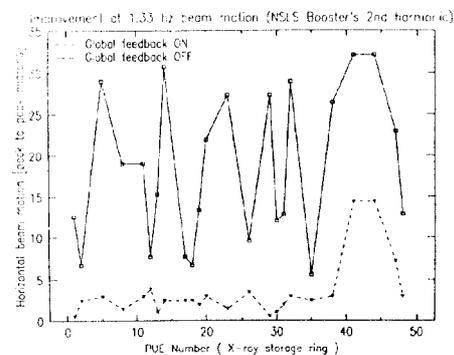
Fig. 4. Horizontal peak-to-peak beam motion at 1.33 hz.
