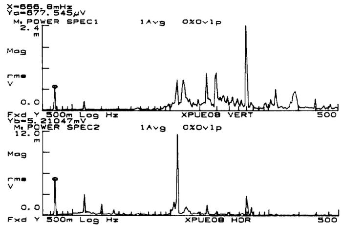
Fig. 3. Spectrum at PUE 08 - 1 mV rms  $\approx$  5.6 microns p-p (measured on 5/3/93 - dry weather conditions)
