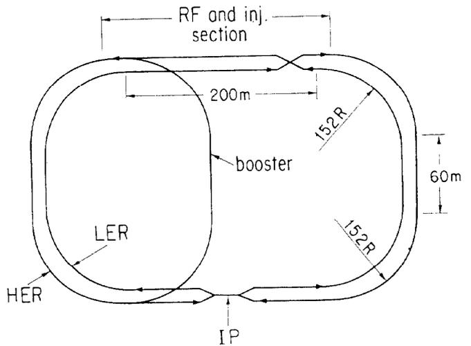
Fig. 1 Layout of booster and B-Factory.
