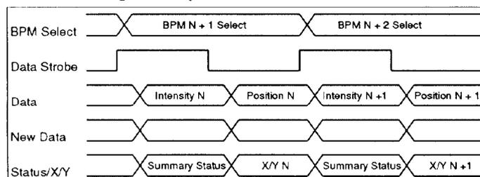
Figure 3. Data Transfer Over the Local Bus
