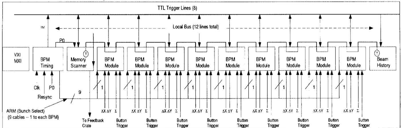
Figure 2. BPM Data Acquisition Block Diagram
