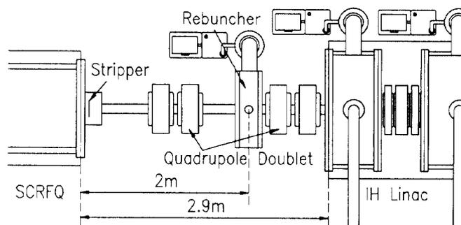
Figure 3. Layout of the stripper section.
