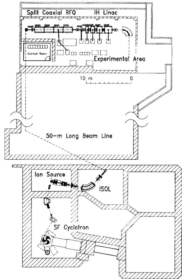
Figure 1. Layout of the radioactive-beam acceleration facility.
