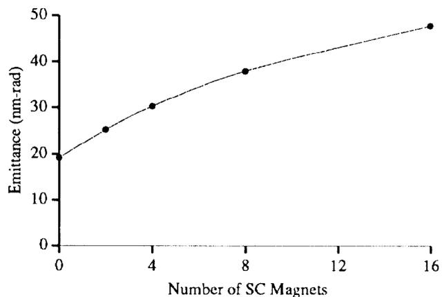
Figure 5. Emittance increase with number of superconducting dipoles.
