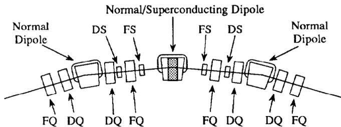
Figure 1. Sketch of TBA unit cell
