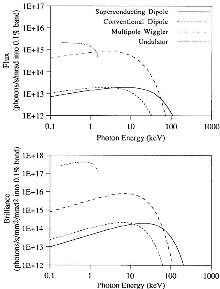
Figure 3. Flux and brilliance of sources in DIAMOND including output from representative insertion devices.
