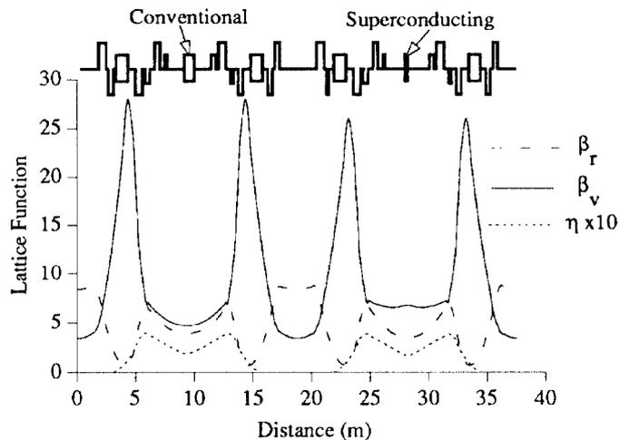
Figure 4. Matched lattice functions in DIAMOND
