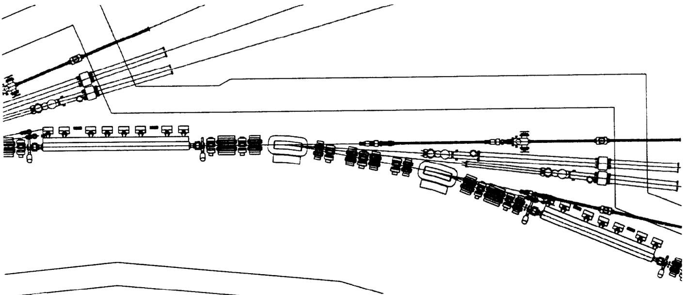
Figure 2: Section of the storage ring. The straight sections on both sides of the achromat will accommodate Undulators and Wigglers. Synchrotron Radiation beamlines are indicated.
