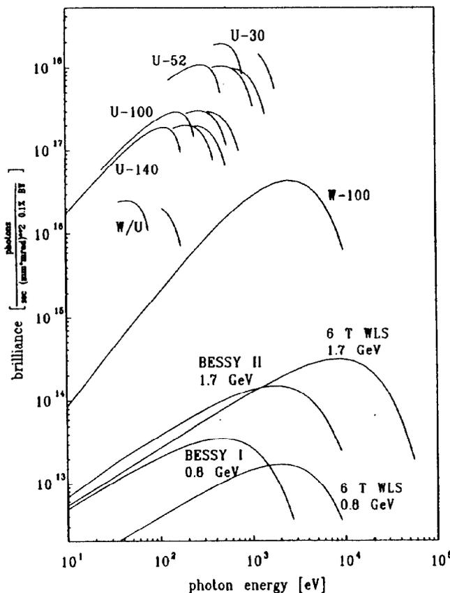
Figure 3: Brilliance of radiation from insertion devices at BESSY II compared with radiation from dipoles and with the 0.8 GeV BESSY I synchrotron radiation source.
