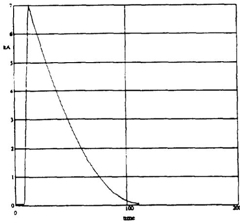
Figure 6 - Current Waveform for Test at 7 kA
