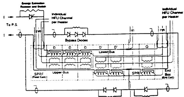
Figure 1 - ASST Phase I Electrical Circuit
