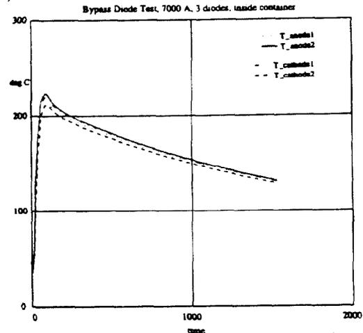
Figure 7 - Temperature Profile vs Time for 3-Diode Assembly at 7 kA
