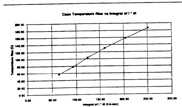
Figure 5 - Temperature Rise at Hottest Spot in Assembly
