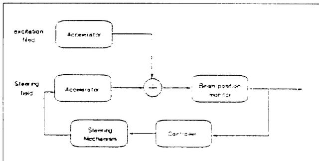
Figure 1. Linear model of beam feedback system.
