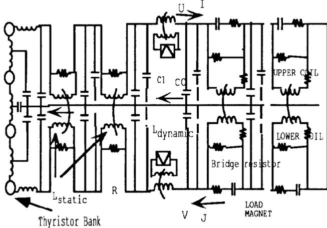
Fig.1 Equivalent circuit of the power supply system
