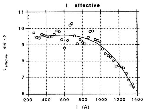
Fig.4 Excitation dependence of Quadrupole Inductance
