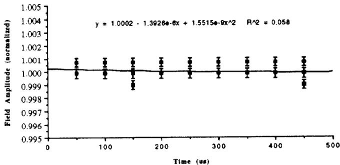
Figure 5. DTL1 Field Amplitude Flatness without beam
