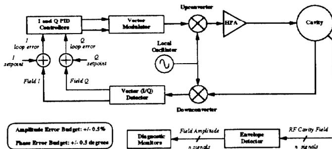
Figure 1. Block Diagram of the RF Control System
