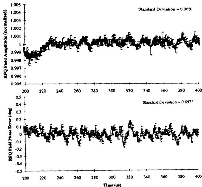
Figure 4. RFQ Field Amplitude and Field Phase without beam
