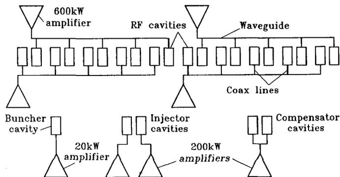
Figure 1: Scheme of RF system for microtron-recuperator.
