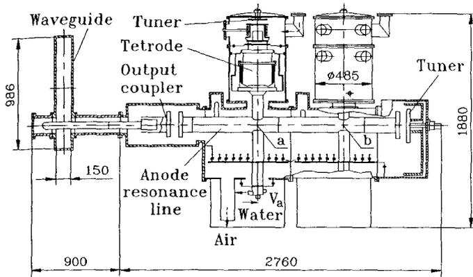
Figure 3: Design of a 2-tube RF power stage.
