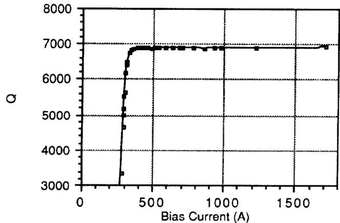
Figure 4. Tuner Q vs. Bias Current.
