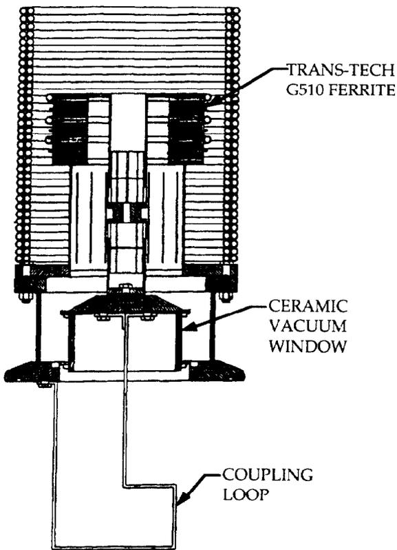
Figure 2. Perpendicularly biased ferrite tuner.
