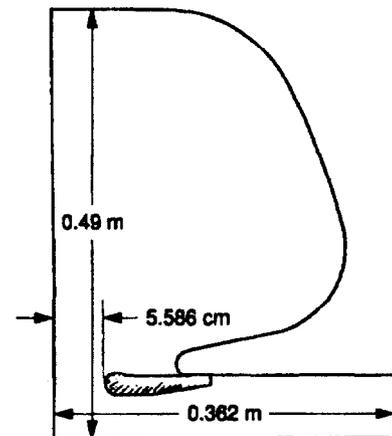
Figure 1. Modified RF Cavity profile with copper extension in nose cone.
