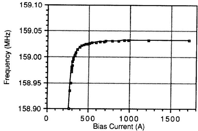
Figure 3. Tuner Frequency vs. Bias Current.
