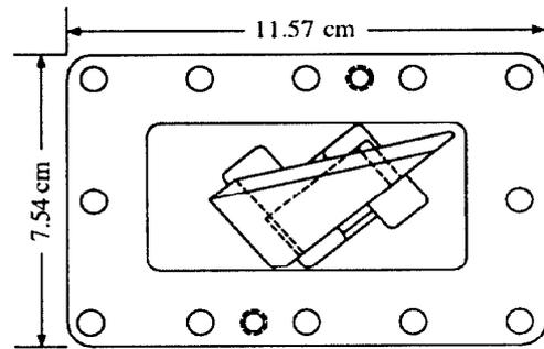
Figure 1. CEBAF's HOM load assembly. The geometry is designed to effectively match to several waveguide modes and over a broad frequency range.
