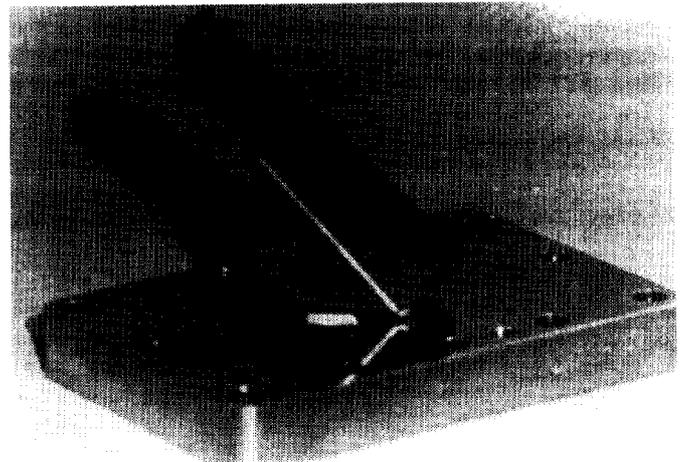
Figure 2. The CEBAF HOM load assembly, with the stainless steel flanges and the brazed lossy ceramic parts. The load is only 7 cm long, thanks to the high dielectric constant of the absorber material.
