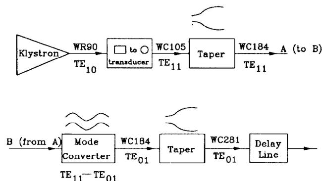
Figure 1. The proposed transmission modes, waveguide size, and conversion sequence for binary pulse compression system at 11.4 GHz operating frequency.
