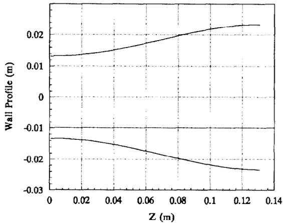
**Figure 2.** The waveguide profile of an optimized 11.4 GHz  $TE_{11}$  uptaper with input and output diameter of 2.67 and 4.67 cm respectively.
