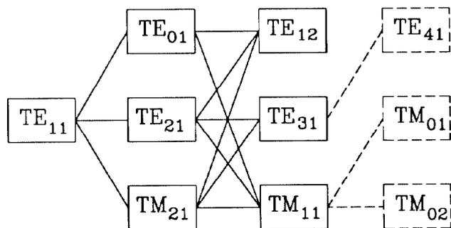
**Figure 3.** Coupling diagram of a  $TE_{11}$ - $TE_{01}$  single plane serpentine mode converter at 11.4 GHz with a diameter of 4.67 cm.
