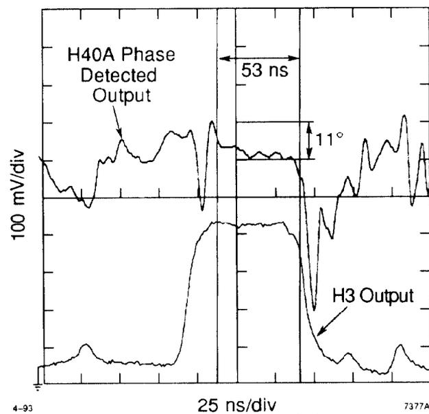
Figure 5. Amplitude and phase of the combiner output pulse.
