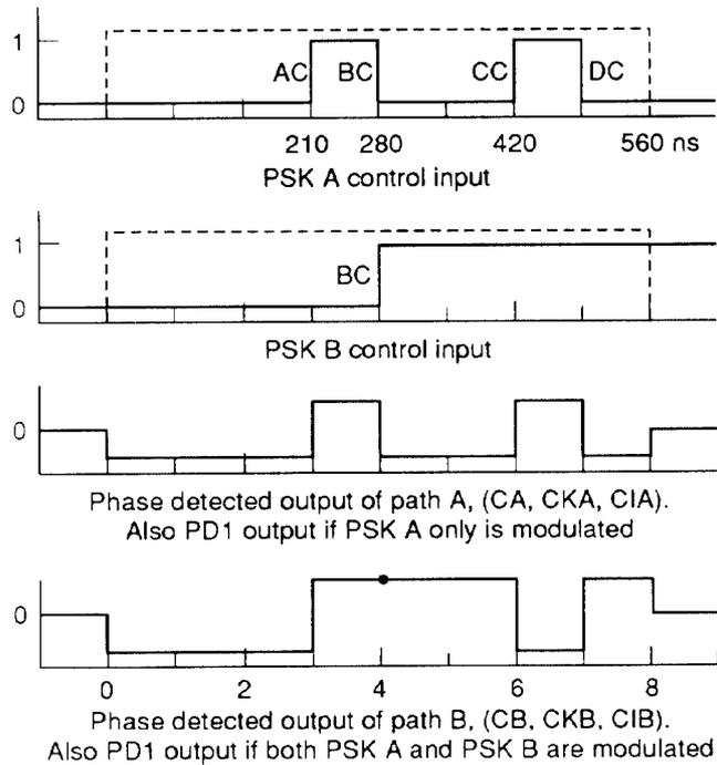
Figure 3. Three-stage BPC modulation (horizontal unit = 70 ns).
