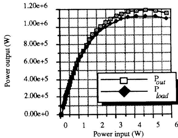
Figure 3. Power transfer of the klystron with cathode current of 28 A.
