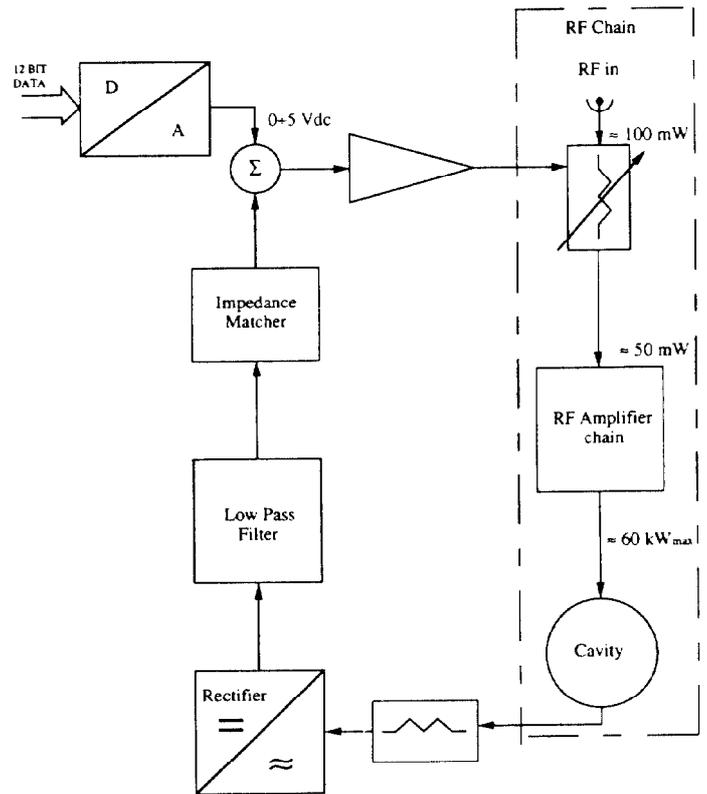
Fig.5 Block diagram of the amplitude loop
