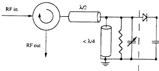
Fig. 4 Schematic drawing of line type phase shifter
