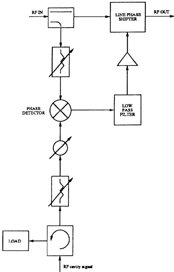
Fig. 3 Block diagram of the fast phase loop
