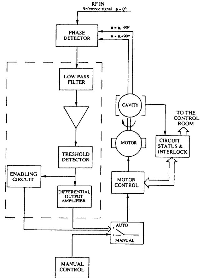
Fig. 2 Block diagram of the mechanical tuning loop
