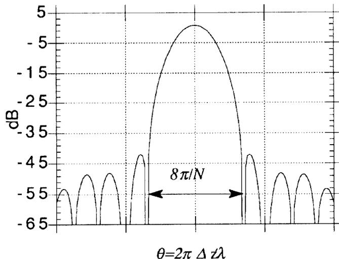
Figure 2. Hamming window impulse response
