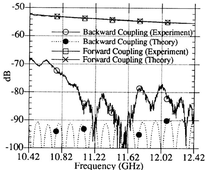
Figure 4. Comparison between theoretical and experimental coupling for the operating mode (TE<sub>01</sub>)
