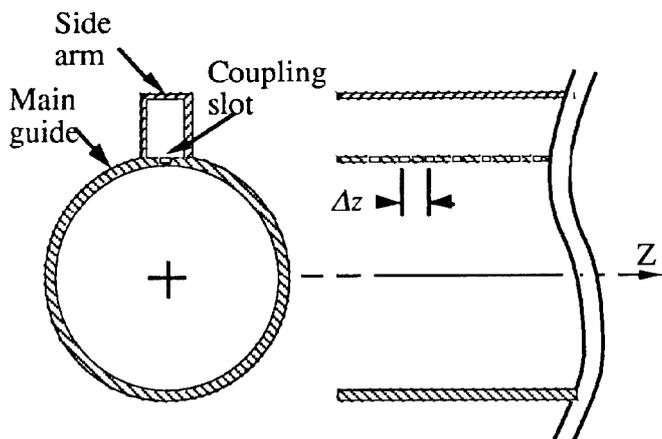
Figure 1 Schematic diagram of the basic coupler geometry
