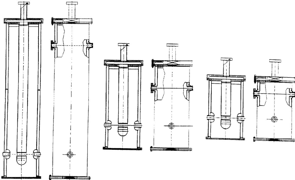
Figure 1: The 80, 160 and 240 MHz niobium resonators.
