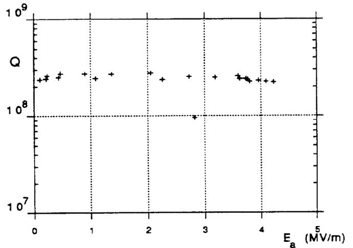
Figure 3: The 80 MHz resonator  $Q$  vs.  $E_a$  curve
