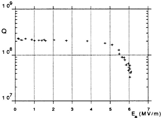
Figure 2: The 160 MHz resonator  $Q$  vs.  $E_a$  curve
