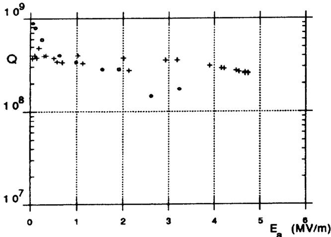
Figure 4: The 240 MHz resonator  $Q$  vs.  $E_a$  curves: "o" before high pressure rinse; "+" after high pressure rinse.
