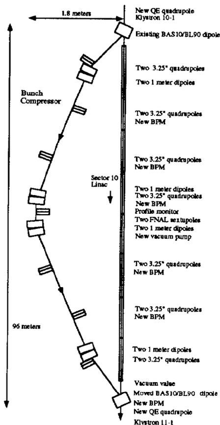
Figure 1 Schematic layout of the short bunch compressor.
