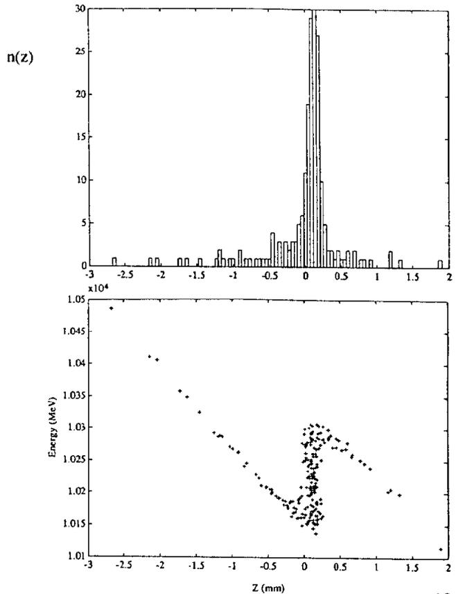
Figure 3 Bunch compression example for  $N = 5 \times 10^{10} e^-$  and  $\sigma_z = 0.08$  mm. The energy versus longitudinal position ( $z$ ) correlation after compression is shown in the lower plot. The longitudinal density distribution is shown in the upper plot.
