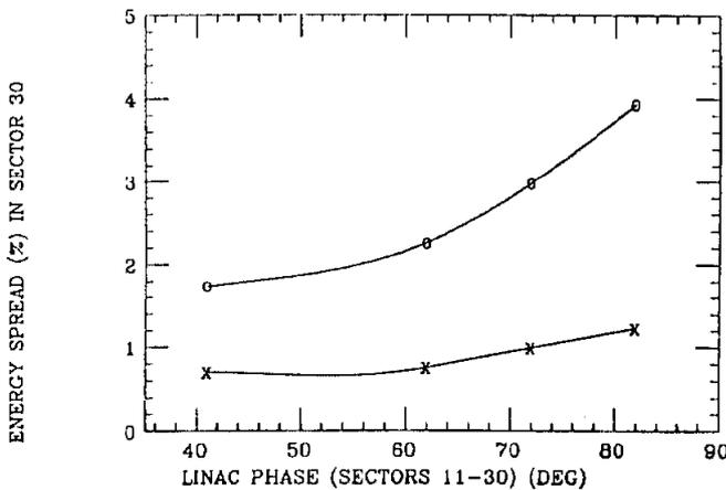
Figure 4 Energy spread at the end of the linac versus linac phase downstream of the compressor. The bunch charge is  $3 \times 10^{10}$  compressed to  $\sigma_z = 0.083$  mm in Sector 10. The (x) points used the nominal longitudinal wakefields in the Sectors 11-30. The (o) points used twice the nominal wakefields. The final beam energies are 25-35 GeV.
