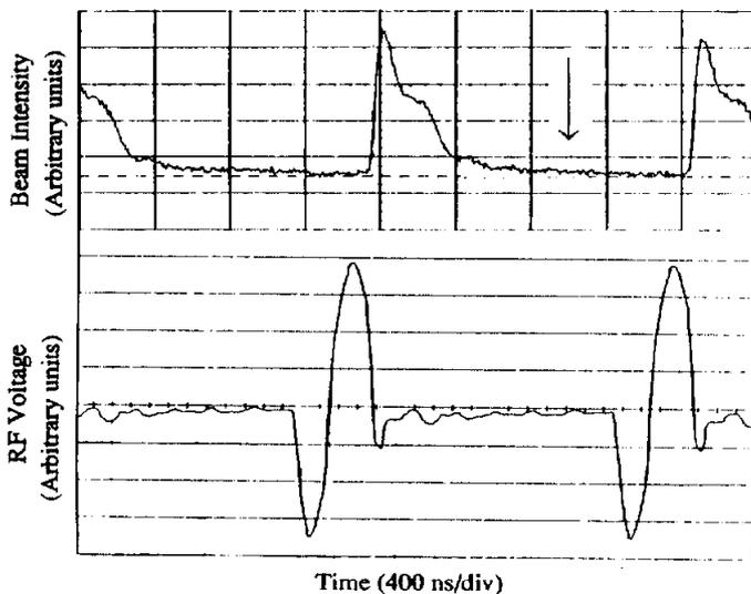
Figure 4. Time distribution of beam in Debuncher after 10-20 seconds of cooling, and the RF wave form.
