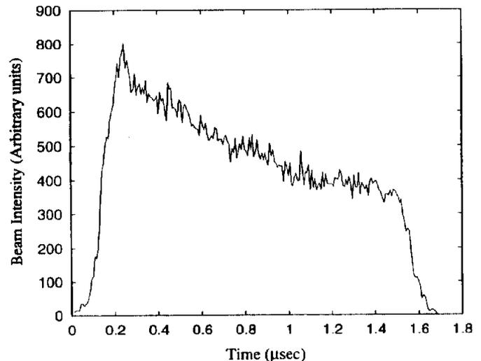
Figure 3. Predicted time distribution of beam injected uniformly into the bucket shown in Figure 2 with no cooling after 2.4 seconds.
