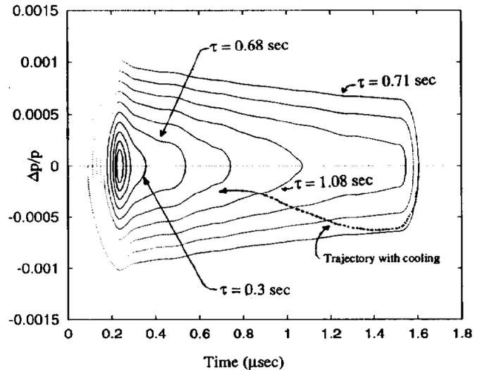
Figure 2. Particle Trajectories in the RF bucket. Contours are 0.01% apart in  $\Delta p/p$ . The synchrotron period is shown for a few trajectories. The dotted arrow is a possible path that a particle may take as it is cooled by the stochastic cooling.
