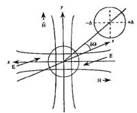
Figure 2. Left circularly polarized deflection cavity, beam deflected upward.
