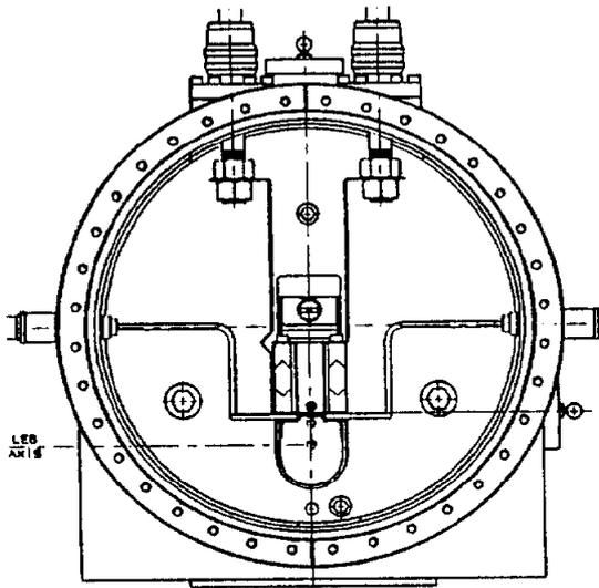
Figure 5. Cross Section of the Short Septum Magnet
