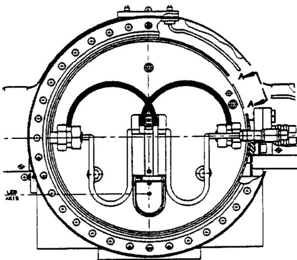
Figure 6. Cross Section of the Long Septum Magnet
