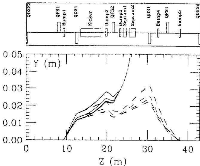
Figure 2. Layout of the Extraction System and the Central Orbit for Bumped and Extracted beam
