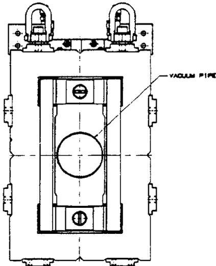
Figure 4. Cross Section of the Bump Magnet
