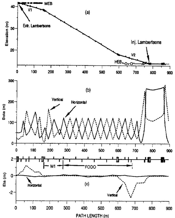
Fig. 2. Layout and lattice functions of the CW line.
