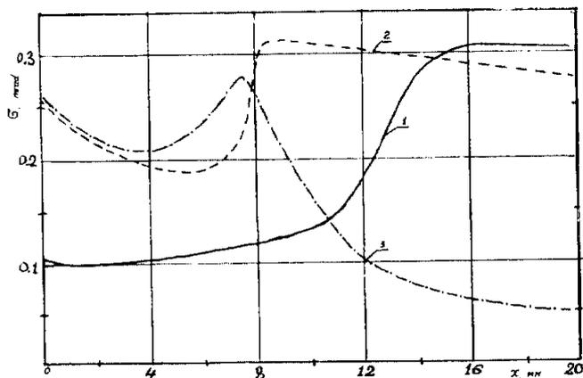
Figure 2: Dependence of the particles angular distribution width on coordinate at steering of the beam onto the thin target. Curves 1,2,3 - as on fig.1.
