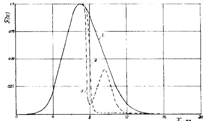
Figure 1: Particle distribution function on maximum coordinate under steering beam onto the thin target. Curve 1 - initial beam into accelerator, 2 - target on negative coordinates, 3 - thin target on positive coordinates.
