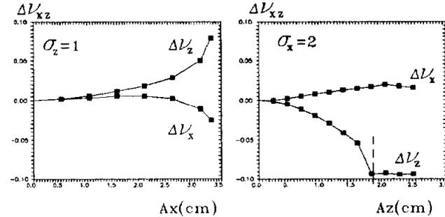
Figure 7: Amplitude dependent tune shift (alternative point).
