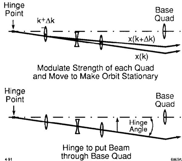
Figure 2. Quadrupole Alignment Procedure
