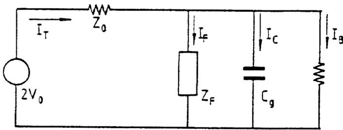
Figure 5 : Induction cell equivalent circuit
