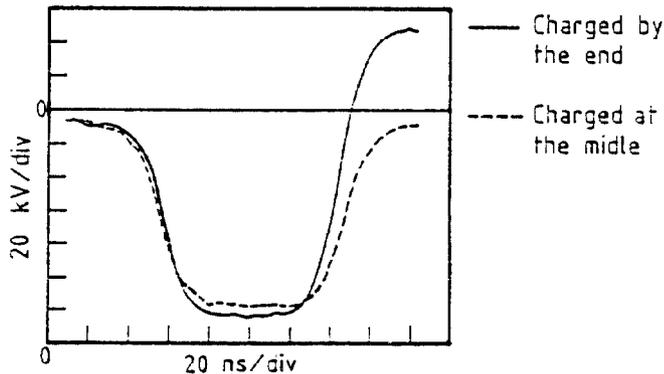
Figure 2 : MAG output voltage
