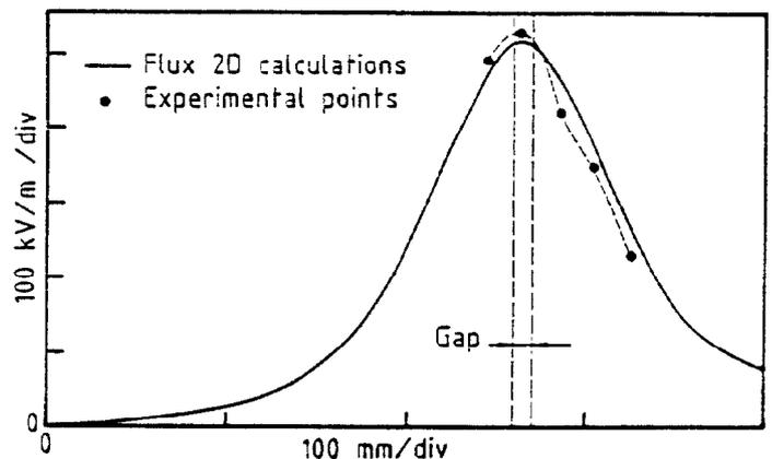
Figure 4 : Electric field profile in beam pipe
