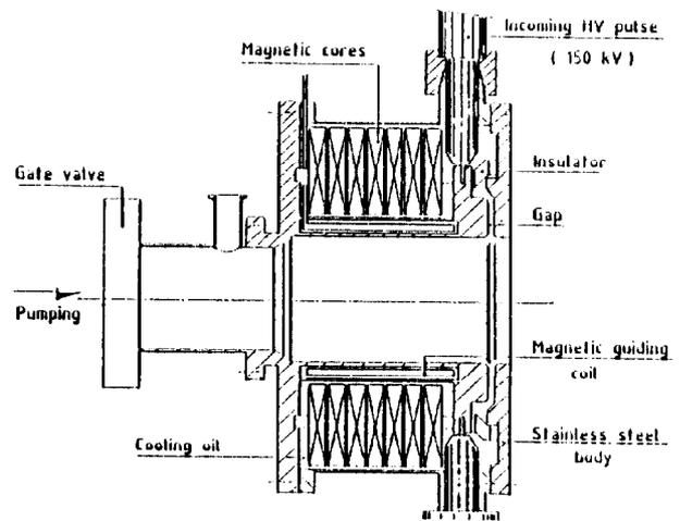
Figure 3 : Prototype induction cell
