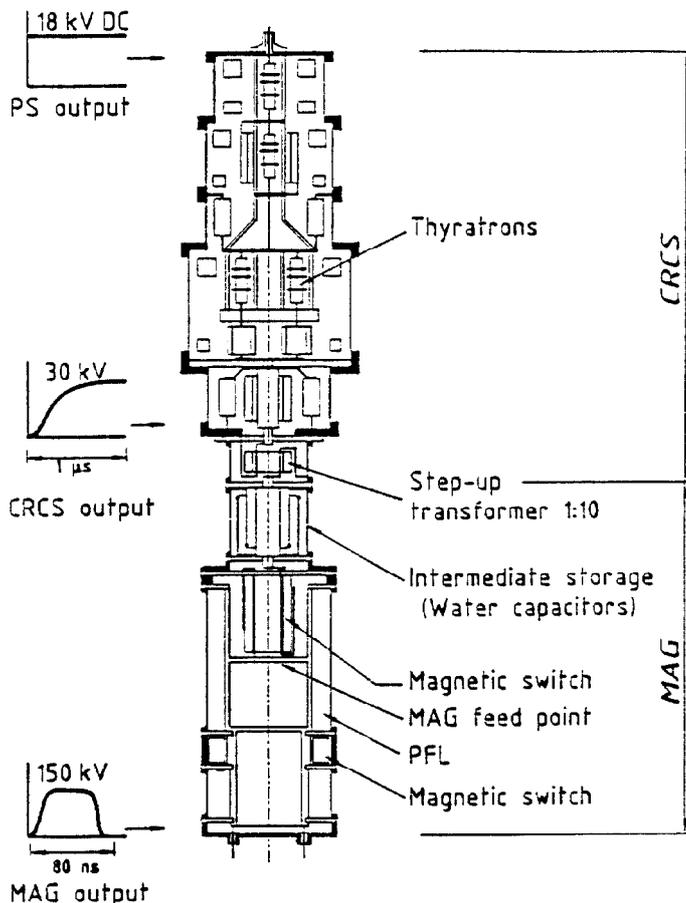
Figure 1 : Cross section of HV pulse generator.
