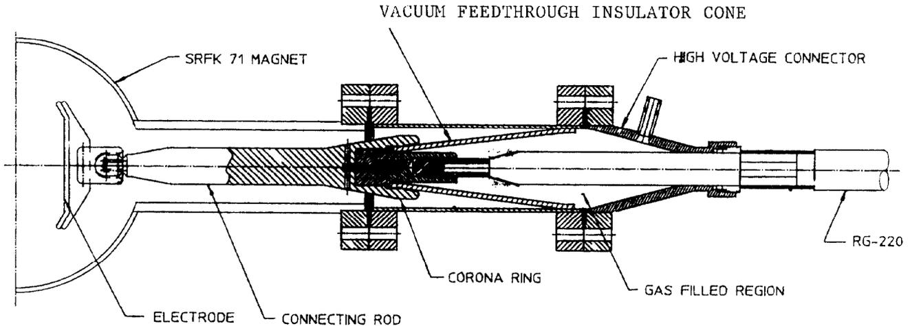
Figure 3: Electrical feedthrough.
