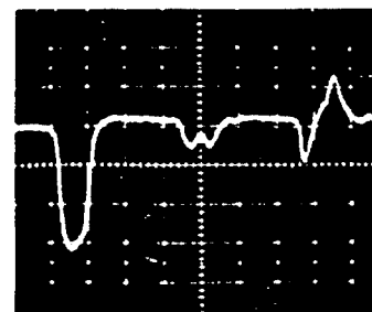
Fig. 4. Measured output voltage waveform for the MAG1D – 28kV input, 126kV peak output.
