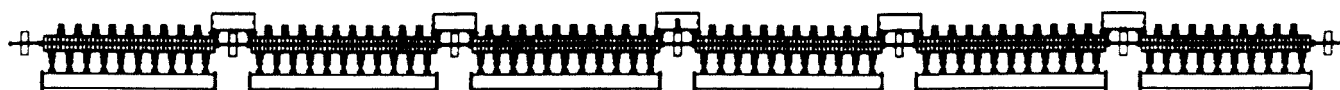
Fig.1 A typical CCL module consists of 6 tanks and 5 bridge couplers. The magnetic quadrupoles between tanks and the vacuum manifolds are also shown.
