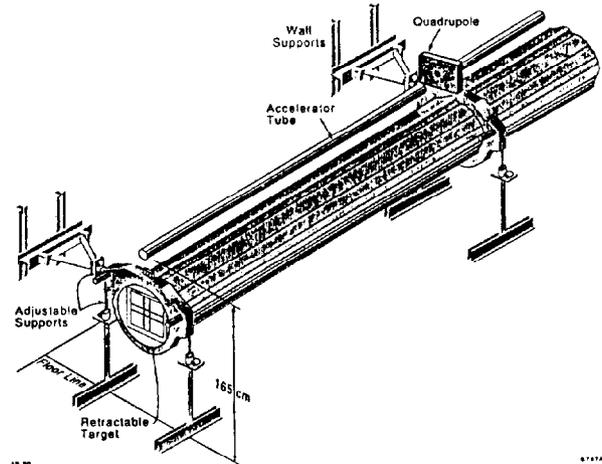
Fig. 1 Support girder for the SLC Accelerator
