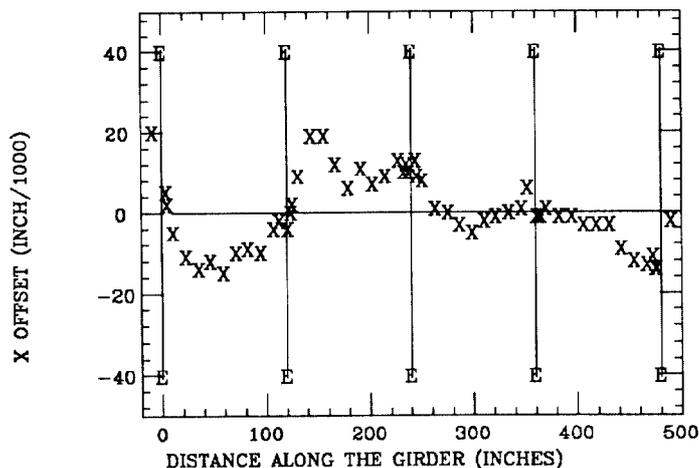
Fig. 4 Measured displacements of an accelerator structure measured every 30 cm. The symbols 'E' refer to the ends of the 10 ft assembly sections.
