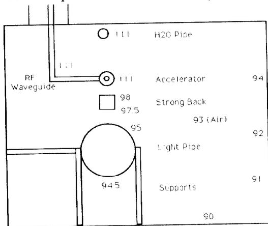
Fig. 5 Typical temperature measurements in the Linac tunnel.
