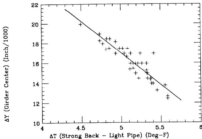
Fig. 8 Measured vertical girder bowing from gradient changes.
