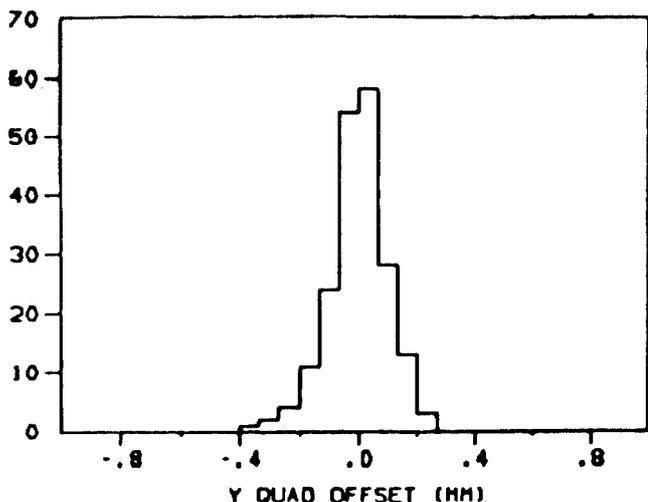
Fig. 3 Vertical residual quadrupole offsets after beam-based alignment.
