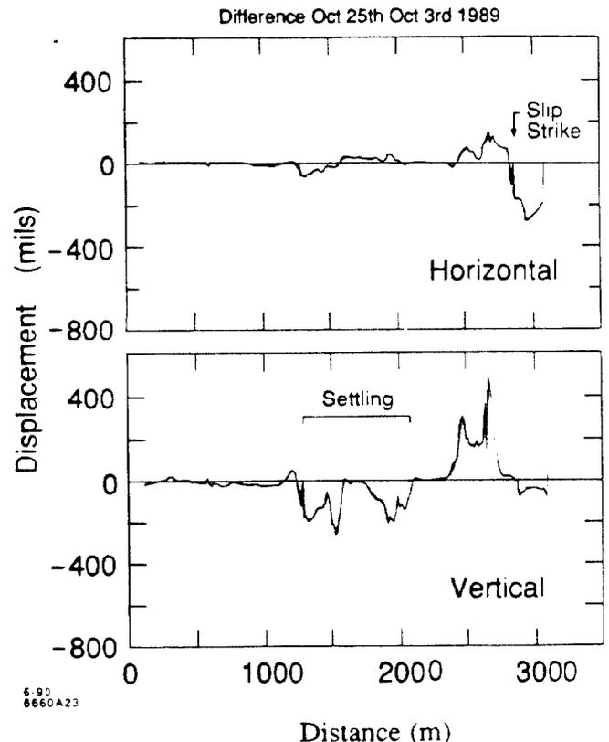
Fig. 2 Observation from the laser alignment system of the settling and shifting of the accelerating structures from the October 1989 earthquake.
