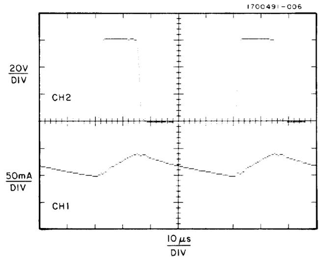
Figure 4. Switching waveforms from a CESR bipolar chopper operating at 6.25 Amps. CH1 is the voltage across the magnet and CH2 is the AC coupled magnet current ripple.
