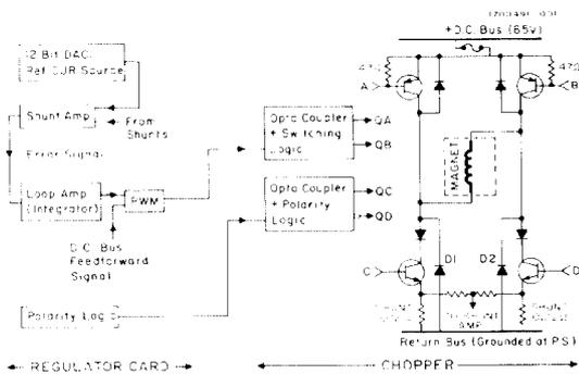
Figure 3. CESR bipolar shunt regulated chopper power supply block diagram.
