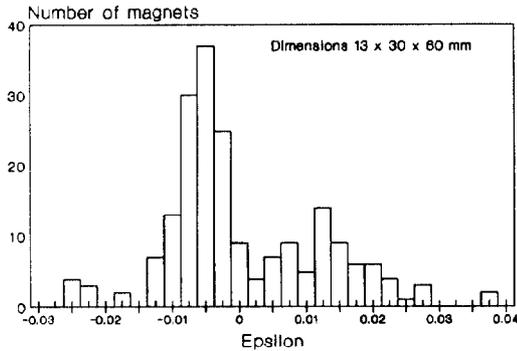
Fig. 5 - Measurements of strength on 200 magnets.
