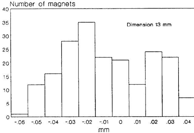
Fig. 3 - Deviation from the nominal dimension (200 magnets).
