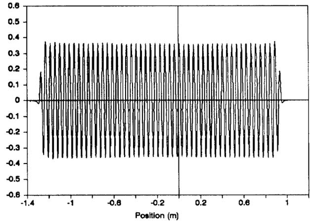
Fig. 7 - Measurements of B (T) along the mechanical axis.
