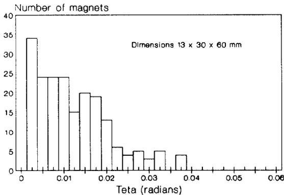
Fig. 6 - Measurements of angular deviation on 200 magnets.
