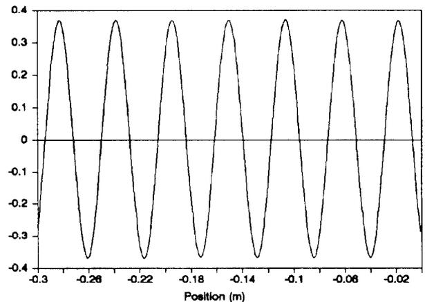
Fig. 9 - Fine measurement of B(T) at the center (mech. axis).
