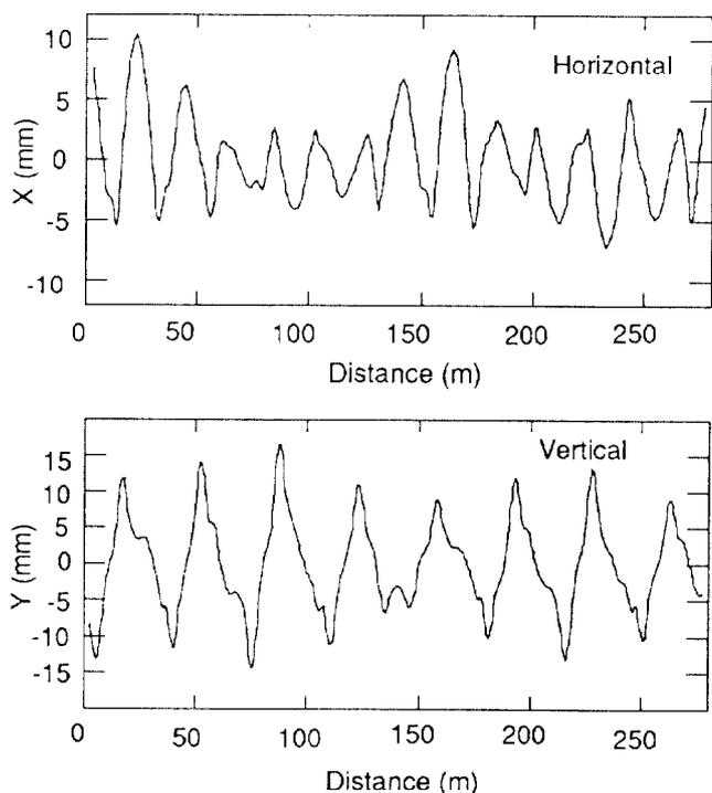
Figure 4: Closed Orbit Distortion Before Correction
