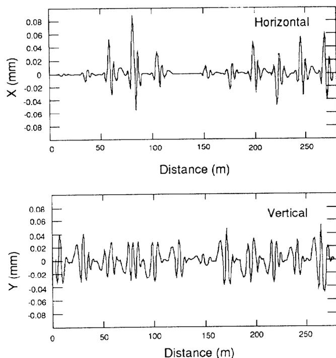
Figure 5: Closed Orbit Distortion After Correction
