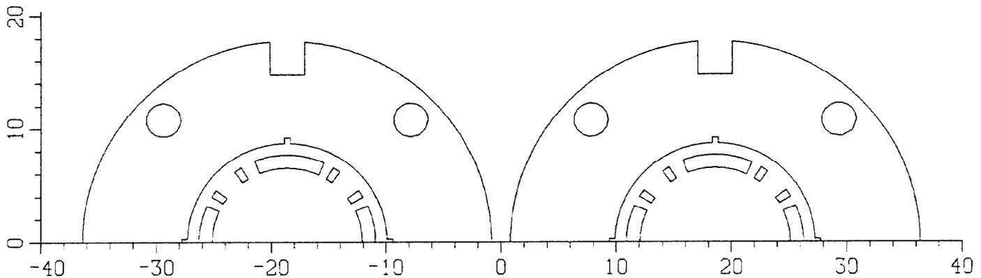
**Figure 2:** Cross section of the top half of the two side by side 130 mm aperture RHIC insertion quadrupoles as placed in the lattice when the separation between the two is minimum.
