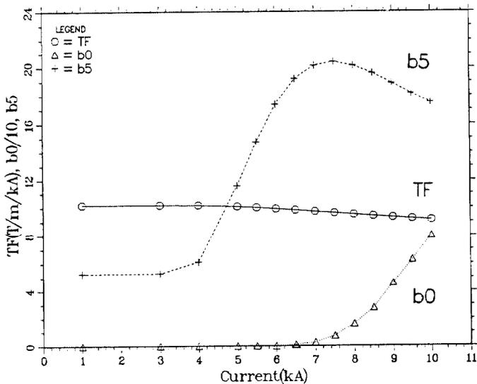
**Figure 3:** Transfer function,  $b_0/10$  and  $b_5$  as a function of current in the RHIC insertion quadrupoles when two of them are placed side by side and are at their minimum distance in the lattice. In this case the two quadrupoles have the same currents.
