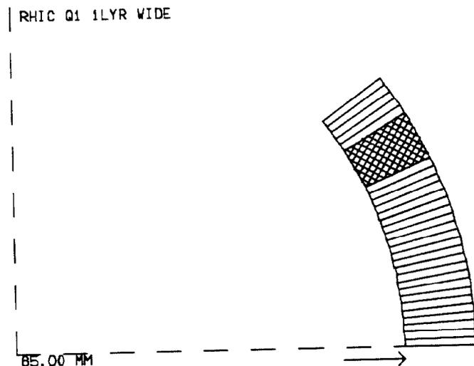
Figure 1: Cross section of the coil for RHIC insertion quadrupoles.
