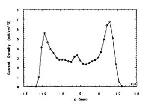
Fig. 2 Measured beam current density distribution vs. radial position. Upper (lower) figure refers to the new (old) source.
