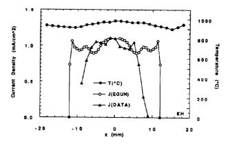
Fig. 6 Test stand measurements of the current density profile J(DATA) compared with EGUN simulation J(EGUN), and the temperature profile taken at the emitter surface.
