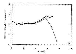
Fig. 4 5 mA beam current density at point of injection into first quadrupole of matching section. Comparison between experiment (Δ) and EGUN code (•).
