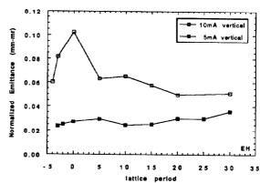
Fig. 5 mA and old 10 mA beam r.m.s. normalized transverse emittance vs. lattice period along MBE-4. The matching section corresponds to lattice periods -4 through 0.
