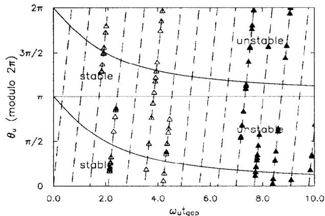
Figure 1: Stability region as a function of  $\theta_u$  and  $\omega_u t_{gap}$ . The closed triangles (vertical) and open triangles (horizontal) correspond to the operating points at 50 'random' places in a CESR-B lattice.
