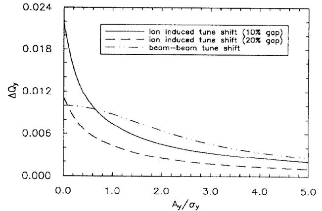
Figure 3: vertical tune shift vs. vertical amplitude
