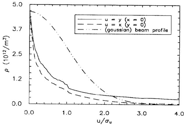
Figure 2: Ion density for a 10% gap. The gaussian beam profile shown for comparison has been normalized to be the ion density at  $x = y = 0$
