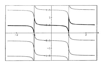
Figure 1 Microwave stability at transition, illustrated by a family of curves representing the phase factor,  $F_n(\omega)$ , in units of  $\pi$ , plotted versus  $x = \omega/\omega_r$ .
