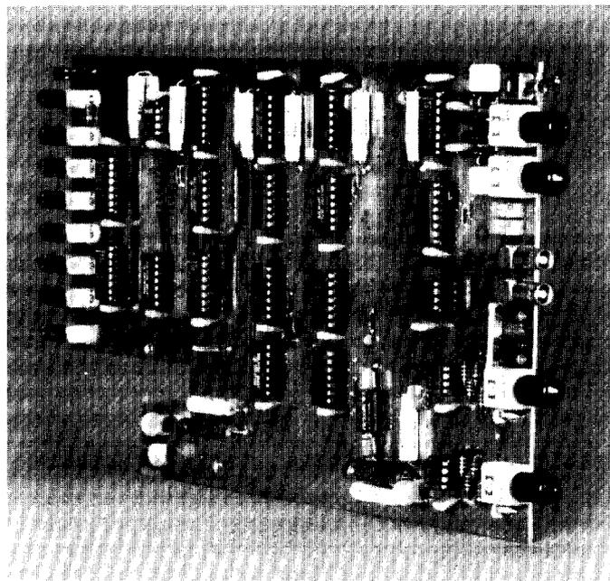
Figure 3. Typical fiber optic repeater. Pairs of optic transmitters and receivers are mounted at the front top and bottom of the repeater board. Local TTL 50 ohm connections are made at the rear of the repeater by means of Lemo style connectors.
